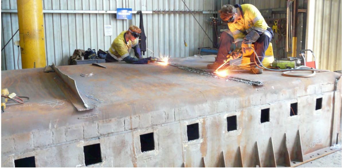
Figure 1: Pot shell repair at Kempe Engineering, George Town
