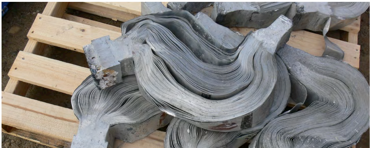
Figure 13: Examples of pot shell "tails" previously discarded and now recycled at Kempe Engineering, George Town
