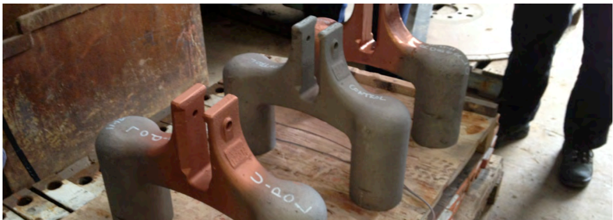
Figure 12: Weld through primer trials for anode rod gussets at CPT Engineering
